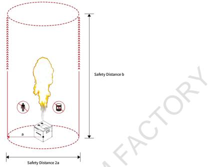
The uFlamer Gasboom safety isolation zone (show as above) is a cylindrical three-dimensional space with safety radius around machine (a) and safety distance at firing direction (b). For safety distance at firing direction equals to maximum firing height+2m. No person and flammable materials are allowed to stay inside the safety isolation zone when flamer was armed. Unauthorized persons and objects are strictly prohibited from entering.
